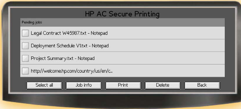
Figure 1. Print jobs are stored on the HP LaserJet MFP hard disk drive (HP Access Control Secure Print Express) or the pull print server (HP Access Control Secure Pull Print) until the document owner authenticates on the MFP.
