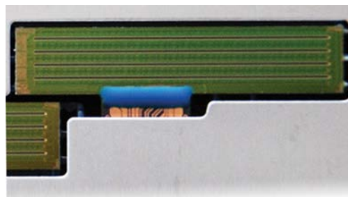
Figure 8. Detail of an HP Thermal Inkjet die
