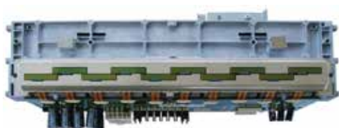
Figure 7. PageWide writing engine assembly, bottom view
