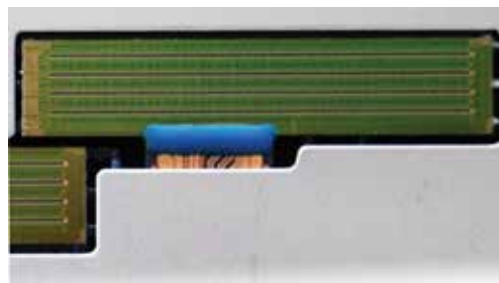
Figure 8. Detail of an HP Thermal Inkjet die
