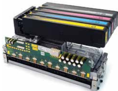
Figure 5. On-axis PageWide writing engine assembly
