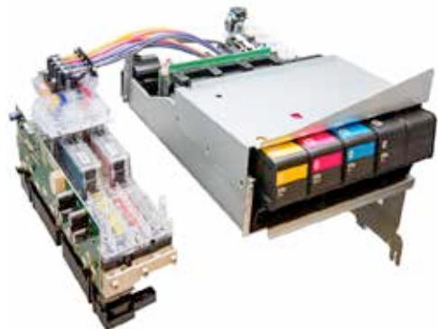
Figure 6. Off-axis PageWide writing engine assembly
