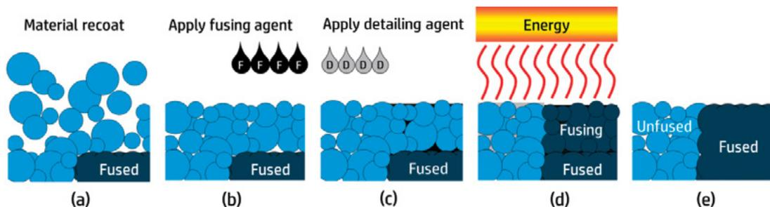
The material is recoated across the work area as shown schematically in Figure 2a.
