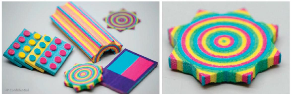
The long-term vision for HP Multi Jet Fusion™ technology is to create parts with controllably variable—even quite different—mechanical and physical properties within a single part or among separate parts processed simultaneously in the working area. This is accomplished by controlling the interaction of the fusing and detailing agents with each other, with the material to be fused, and with additional transforming agents.
