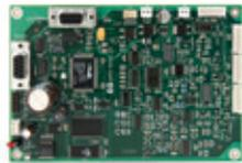
**IDS interface board.** This electronic board mounts on the modular ink supply stall assembly and enables access to ink level sensing and other advanced ink cartridge features. Each board controls up to four modular ink supply stall assemblies. Incorporating this board into the design increases printing system functionality and reliability. For example, it can confirm ink cartridge compatibility, deliver "low ink" warnings, or enable hot swapping of ink cartridges.
