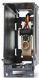
**Modular ink supply stall assembly.** This component provides easy mounting of the bulk ink cartridge, as well as proper electrical and mechanical connection every time the cartridge is changed. When multiple ink cartridges are required, simply snap together as many modular ink supply stall assemblies as needed.
