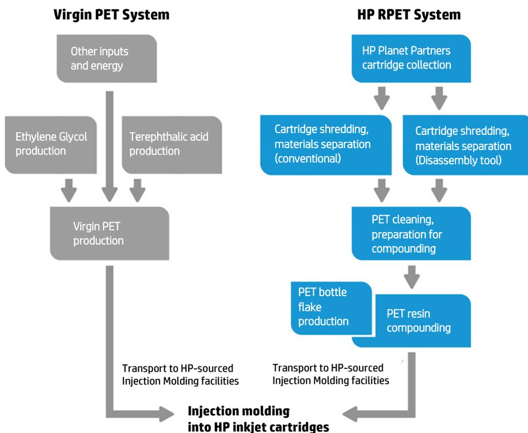
The virgin PET system represents the cradle-to-gate of the sourced PET in HP ink cartridge manufacturing plants worldwide. This system starts at the production of PET precursors and manufacturing of PET resin, and continues through the distribution of the PET resin to injection molding facilities near final cartridge manufacturing.
