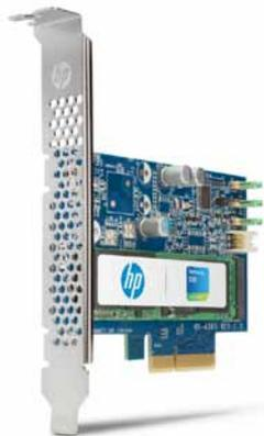
HP Z Turbo Drive featuring Samsung M.2 PCIe SSD technology
