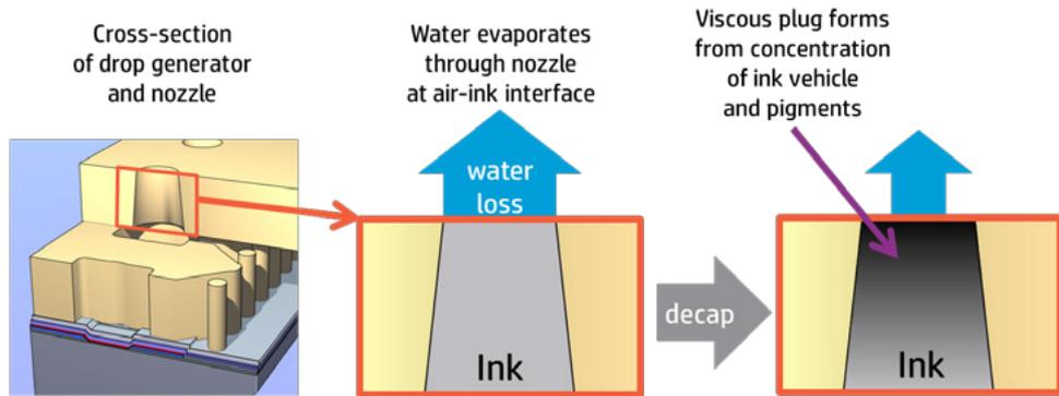
Designing an ink that dries quickly on the print—but doesn’t dry out in the nozzles—is one of the conflicting requirements for inkjet inks. With sustained printing, a pagewide printhead may be decapped for minutes at a time.
