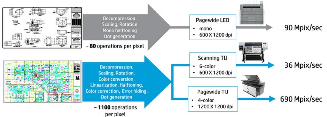
The modular architecture of the image processing pipeline for HP Pagewide XL Printers is shown schematically in Figure 8. Wider (or narrower) printbars can be built by adding (or removing) print module controllers. As with the printhead and ink supply modules, the image processing pipeline is modular and scalable along the printbar. By adding hub controllers for each printbar, multiple printbars can be supported in future product platforms.
