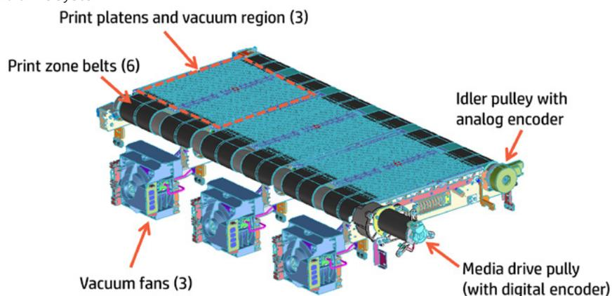
The belts are driven by a fixed drive pulley on the output side of the print zone using a DC servo motor with a digital encoder and transmission. The idler pulley on the input side is encoded by an analog encoder, and is pushed away from the drive pulley by four (4) tensioner springs. The pulleys have guiding grooves for the belts to suppress lateral motion.
