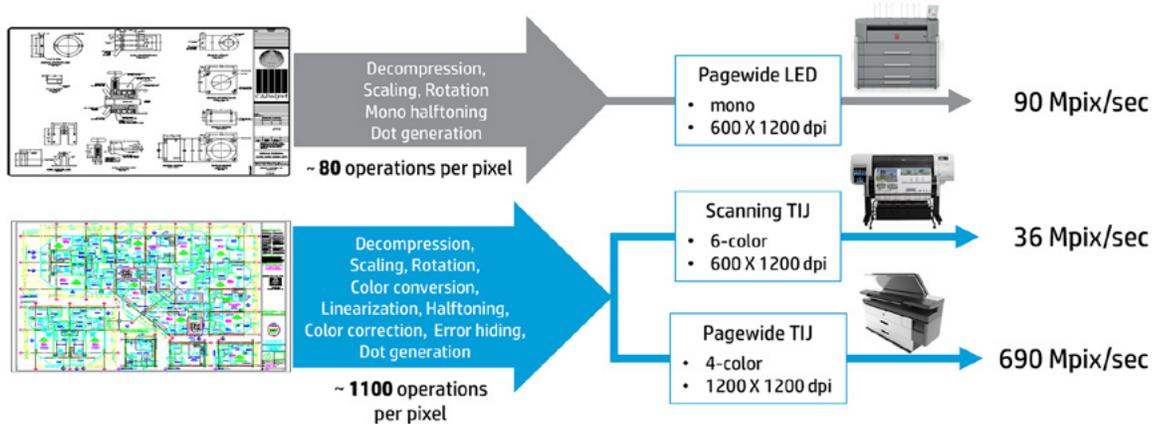
The modular architecture of the image processing pipeline for HP PageWide XL Printers is shown schematically in Figure 8. Wider (or narrower) printbars can be built by adding (or removing) print module controllers. As with the printhead and ink supply modules, the image processing pipeline is modular and scalable along the printbar. By adding hub controllers for each printbar, multiple printbars can be supported in future product platforms.
