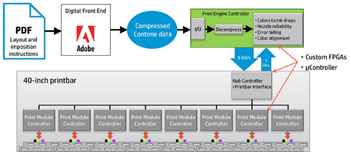
Throughout the image processing pipeline, microcontrollers and custom FPGAs—Field-Programmable Gate Arrays—perform image processing and data management tasks. FPGAs run HP algorithms at speeds up to 190 billion operations/sec.
