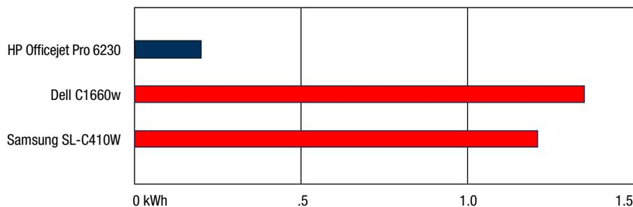
Typical Electricity Consumption is calculated based on each device printing 288 pages per day, with the device spending the remainder of the time in idle and sleep modes after printing is completed. The Yokogawa WT210 power meter is used to measure energy usage during printing and in sleep mode for each device.
