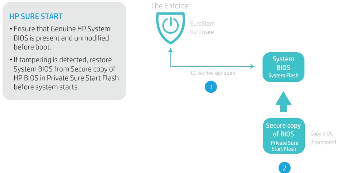
Figure 1. Baseline HP Sure Start overview (applies to HP Elite products equipped with 6th generation AMD processors and higher).
