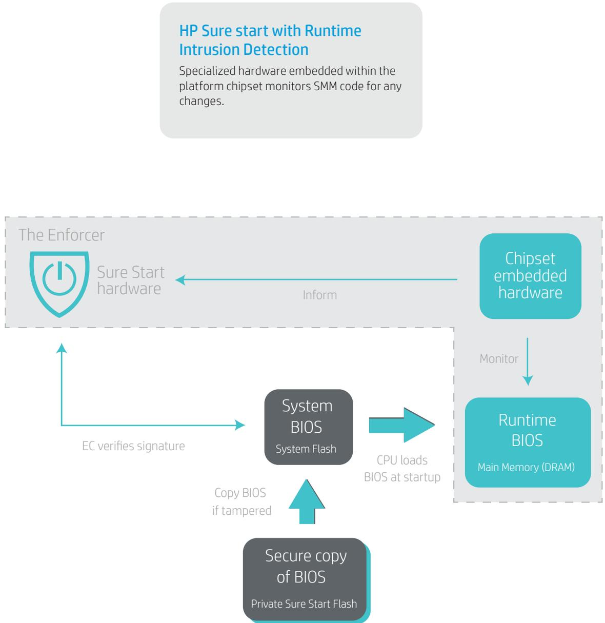
Figure 2. Runtime Intrusion Detection architecture (applies to HP Elite products equipped with 7th generation AMD processors).
