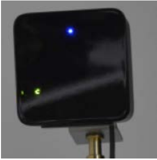
Fig. 3 – Lighthouse from the front. Note the channel indicator in the lower left corner.
