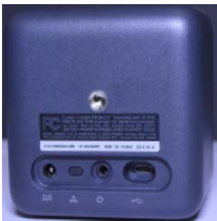
Fig. 4 – Lighthouse from the rear. The centered silver item is threaded receiver for mounting hardware. From left-to-right, the bottom items are: power in, channel button, optical sync cable, and USB port. (for firmware updates).
