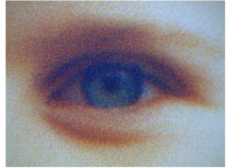
Previous generation HP ink cartridges Colours are blended to create dark areas, sacrificing the dynamic colour range
