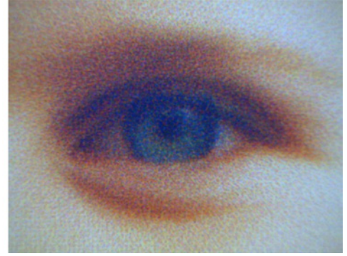
Previous generation HP ink cartridges Colors are blended to create dark areas, sacrificing the dynamic color range
