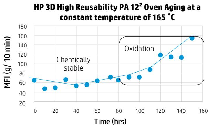
When HP 3D High Reusability PA 12<sup>2</sup> is exposed to 165 °C, the bed temperature in HP's Multi Jet Fusion technology, it takes 80 hours for the material to begin to oxidate.
