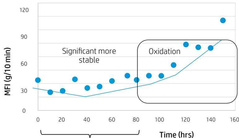
HP 3D High Reusability PA 12<sup>2</sup> viscosity does not strongly change and it can be recycled 20% fresh and 80% reused without degrading the material and consequently not affecting part quality.
