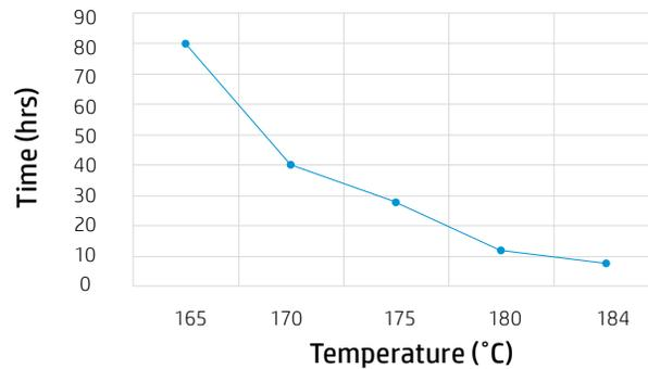
The higher the white powder temperature is, the faster the oxidation takes place.
