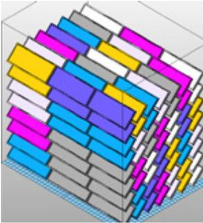
The printed parts are hotter than the white powder. If there is not enough distance between printed parts, the white powder trap between them, gets even hotter than 165 °C probably reaching 185 °C.
