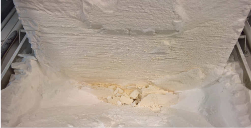
*Example of brown powder in an HP Multi Jet Fusion printed bucket
