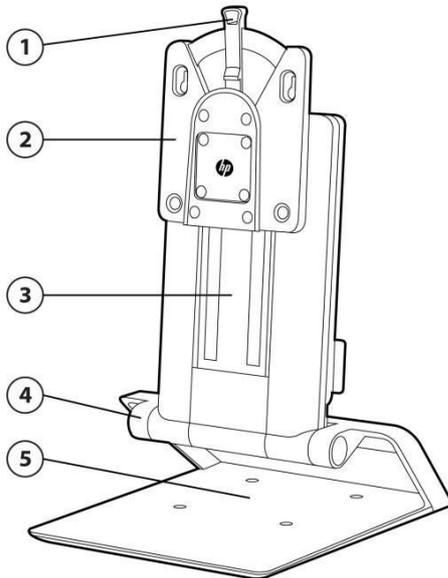
1. HP Quick Release mounting latch
