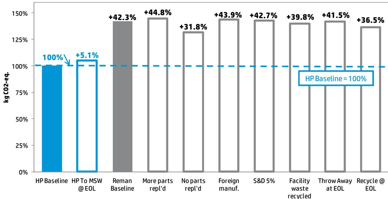
The HP baseline (solid blue) is on the far left, with its corresponding sensitivity analysis to its right. The reman baseline has a dark grey fill with its corresponding scenarios to its right. All results are normalized to the HP baseline (100%), and the percentages shown are the net difference.
