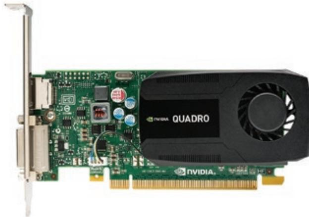
The NVIDIA® Quadro® K420 is a 1 GB DDR3 RAM card designed for professional AutoCAD users.
